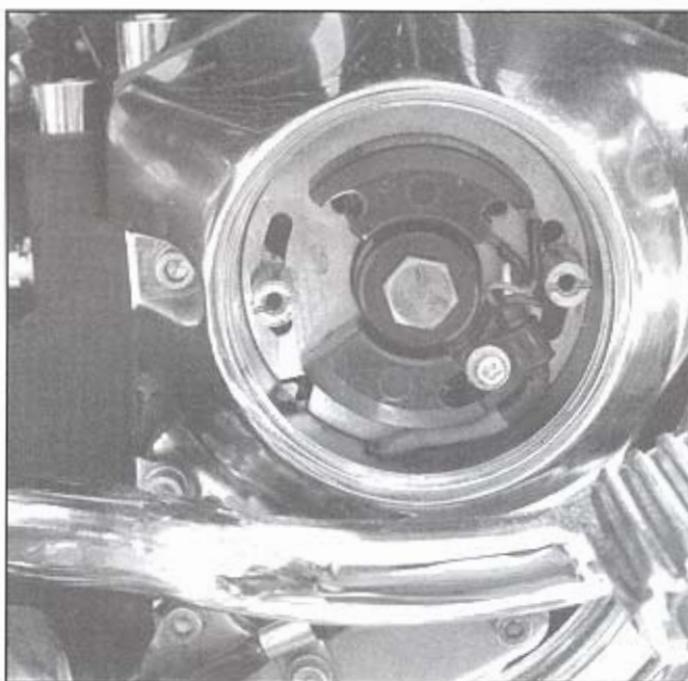
The Dyna "S" single-fire electronic ignition uses a Hall Effect magnetic trigger and a mechanical advance unit for the advance curve. It should be combined with a high-performance coil for maximum performance. Shown is the Dyna single-fire magnetic trigger module.
