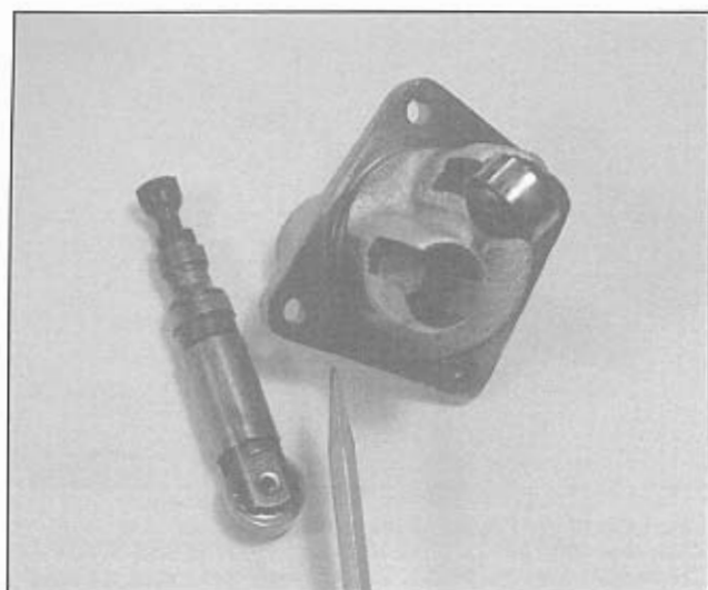
The pencil points to the location of an oil hole in the lifter block that needs to be blocked off when converting from hydraulics to solids. Shown is a Shovelhead lifter block.
