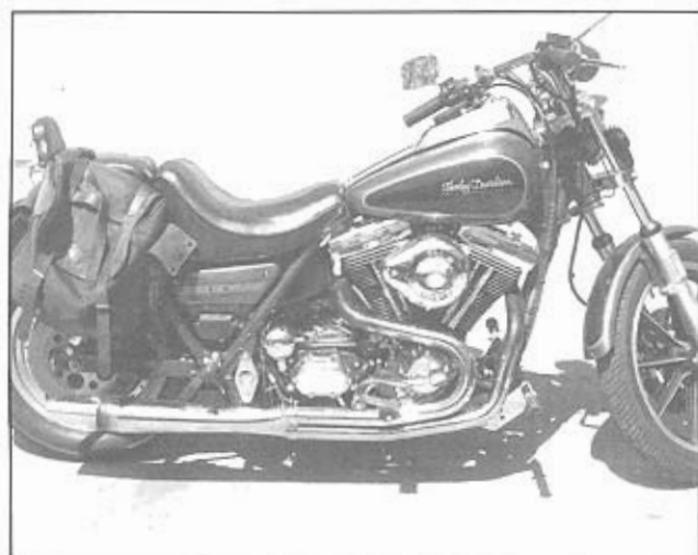
A two-into-one collector uses the low pressure area created by the exiting exhaust gases from one cylinder to help scavenge the other cylinder. Shown is the Thunderheader from Rich Products.
