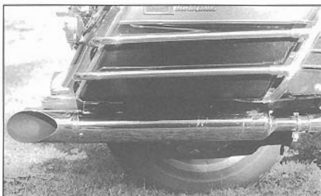
These slip-on touring mufflers are large in volume and offer different end cap designs. The large volume improves exhaust flow while keeping noise down. It also is the reason the touring bikes have more torque than the models with smaller mufflers. The Harley/Kerker touring mufflers use the A-B-C baffle set for silencing. The SuperTrapp version uses diffuser disks.
