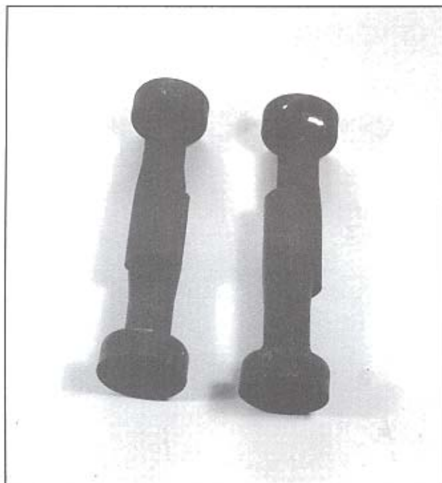
Shown are the "C" baffles used in the Kerker touring mufflers. For racing, you can increase exhaust flow over 300 percent by drilling out the pop rivets and removing these baffles. Don't forget to enrich the carburetor jetting.
