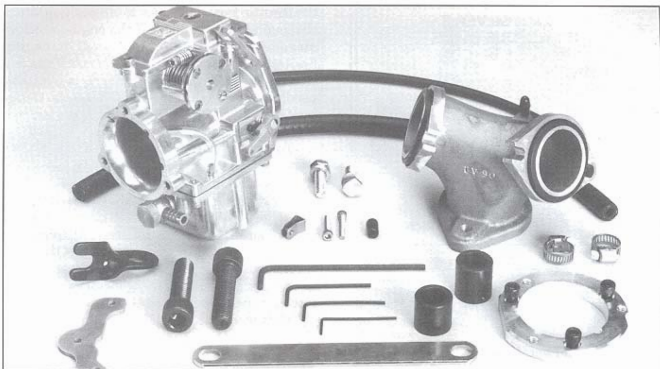
The Qwik Silver II is a high flowing flat slide carburetor that uses one fuel circuit for metering fuel in all rpm ranges. The entire circuit is controlled by one tapered needle, which is available in various sizes. This carburetor is available in 38/40/42mm sizes for Big Twins. High flowing design, simplicity, easy adjustments, and chrome plated die cast body are only some of its benefits. Carburetor kit includes manifold, air cleaner and necessary hardware. Photo courtesy of Qwik Silver II, Inc.
