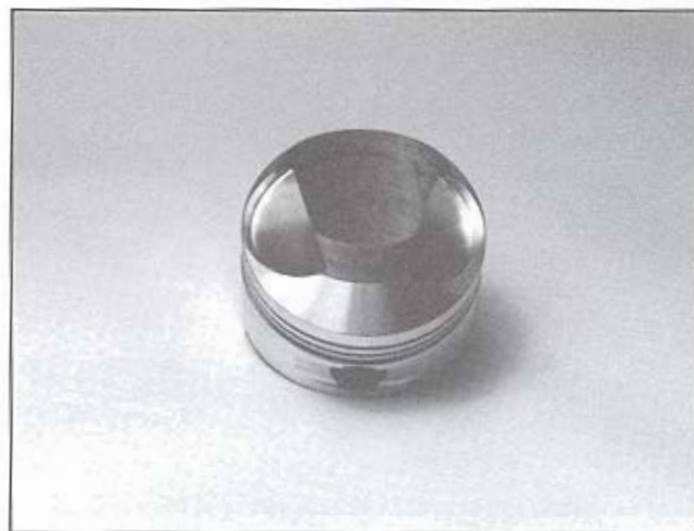
The Axtell 30 degree angle top piston for the Evolution gives about 10:1 compression. It is designed for a single squish band combustion chamber and requires a 30 degree angle cut into the stock chamber's squish ledge. Photo courtesy of Axtell Sales.
