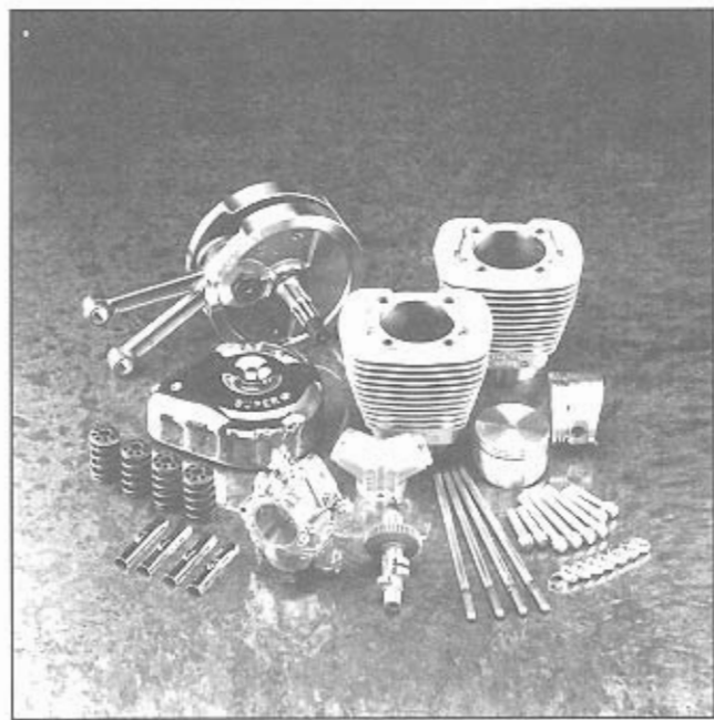
Long stroke flywheels and stroker pistons provide a simple and direct route to increased displacement. Large bore cylinders can be installed along with the stroker flywheels or added later for an even larger increase in displacement. Photo courtesy of S&S Cycle.
