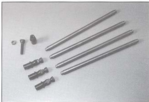
Shovelhead hydraulic lifters easily collapse due to loose tolerances and low oil pressure. S&S Shovelhead Solid Lifter Conversion Kit with non-adjustable pushrods is one remedy for the problem. Photo courtesy of S&S Cycle.
