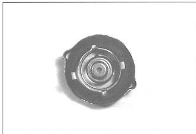
The fuel tank must be vented properly for adequate fuel flow. Notice the additional vent hole drilled near the top underside of the cam style gas cap. This modification is for race track use only.
