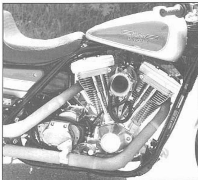
Stepped headers create more energy pulses and can improve cylinder filling. These straight pipes are wrapped with braided ceramic insulation for greater heat retention and higher gas velocity. If you look closely, you can see the pipes have three steps under the wrap. Frank Rayburn on the Neidengard's Cycle Center 80 ci Evo holds the AHRA E Street 1/8 mile record at 6.67 E.T. and 105.10 mph. Photo courtesy of Larry Smith/Handcrafted American Racing Motorcycles.
