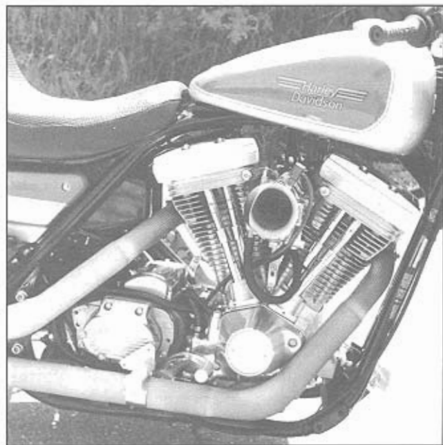
A carburetor with high airflow takes priority over air filtration on a drag bike. Note the large fuel line and deflector shield on the end of the velocity stack. Photo courtesy of Larry Smith/Handcrafted American Racing Motorcycles.
