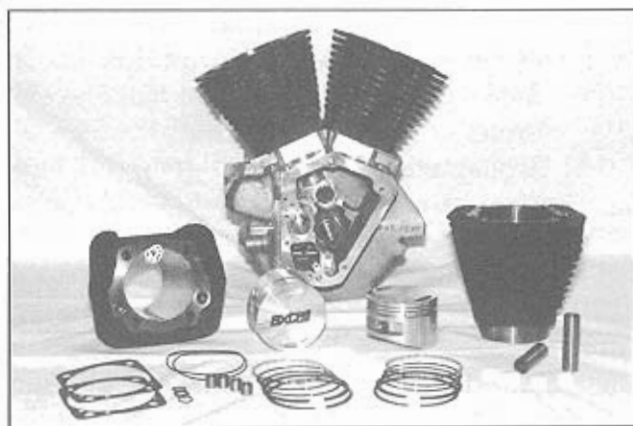
You can increase displacement to 97 cubic inches while retaining the stock stroke by installing 3-13/16" bore cylinders. Shown is Axtell's big bore Shortblock Kit. Photo courtesy of Axtell Sales.
