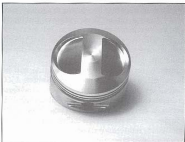
Axtell 30 degree full dome Evolution piston gives about 10:1 compression when used with a bathtub style combustion chamber such as a STD or Branch #4 head. Photo courtesy of Axtell Sales.
