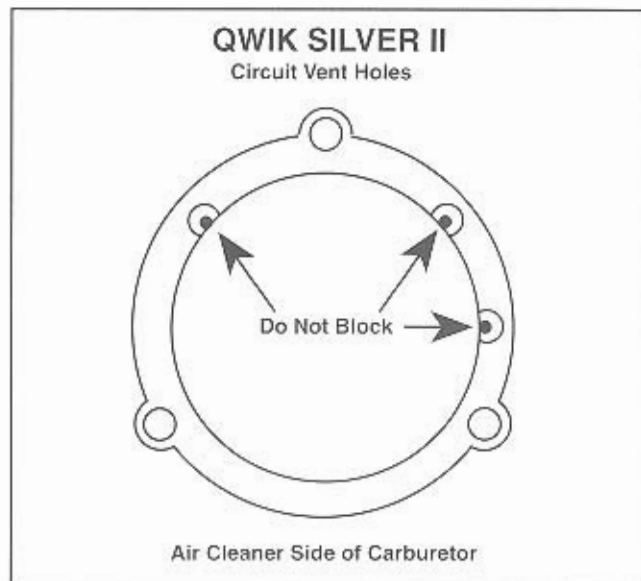
The three circuit vent holes allow atmospheric pressure to enter the fuel bowl area and starter enrichment circuit. To avoid a lean condition, especially at high road speeds, be sure the air cleaner or velocity stack does not block any of the holes.
