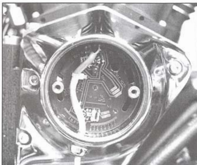
The M.C. Power Arc optical trigger replaces the stock trigger mechanism. The sensor plate includes adjustment slots and a red LED (top center) to simplify static timing.
