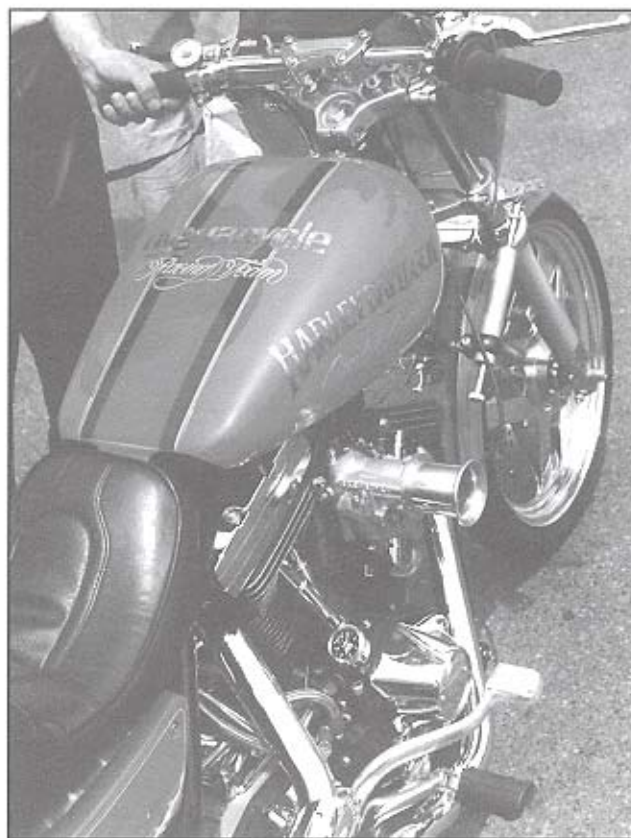
S&S Super B carburetor on Chris Barbarie's beautifully detailed FX. Notice the adjustable air bleed jet on the side of the carb. Chris runs in an ECRA Eliminator class on an 11.30 E.T. index. Photo courtesy of Larry Smith/Handcrafted American Racing Motorcycles.
