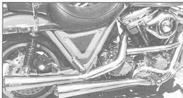
These slip-on mufflers from SuperTrapp are tunable by adding or removing diffuser disks. Randy Diamond's stock stroke 97 ci Evo retains the header crossover pipe and uses SuperTrapp open end caps for more power and sound. Photo courtesy of Great Lakes Cycle.
