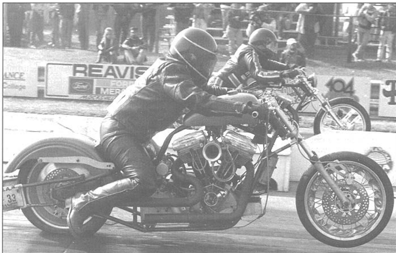
Straight pipes offer maximum exhaust scavenging, which is needed for lots of horsepower and low elapsed times in drag racing events. Photo courtesy of Larry Smith/Handcrafted American Racing Motorcycles.
