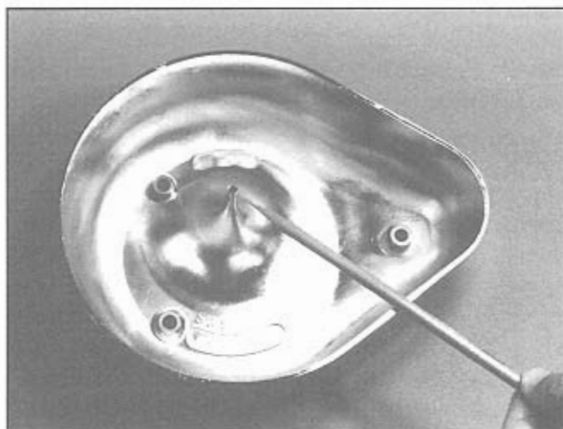
Notice the radiused entryway and air directional cone on the inside of the S&S air cleaner. This design increases airflow by capturing air and smoothing it out while directing it into the carb's throat.
