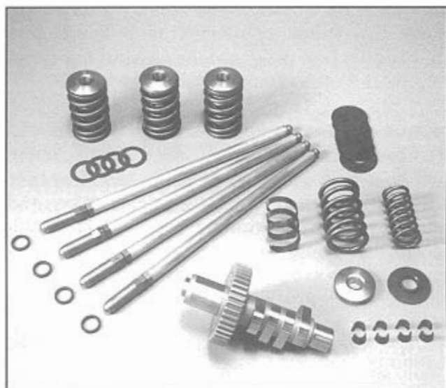
Kits are available that not only include a cam, but also all necessary valvetrain components for easy cam installation. The four small washers at the bottom ends of the pushrods convert Evolution hydraulic lifters to solid action when the engine is at high rpm. Shown is an S&S Evolution cam kit with titanium spring collars and Hydraulic Lifter Limited Travel kit. Photo courtesy of S&S Cycle.
