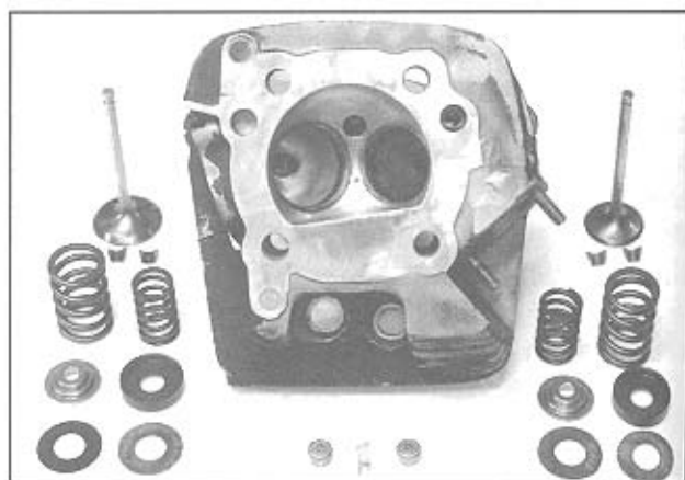
Stock D-shape Evolution combustion chamber has a 90 degree squish ledge on one side and the spark plug on the other. This chamber is much smaller and more turbulent than the Shovelhead chamber, resulting in faster and more complete combustion. This head was reworked by Carl's speed shop. Photo courtesy of Carl's Speed Shop.
