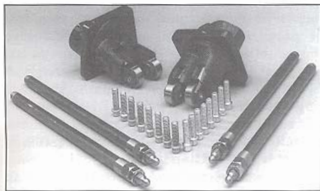
The Velva-Touch Lifter Kit eliminates hydraulic lifter pump up and maintains zero valve lash to over 7000 rpm. Machined to close tolerances, these lifters eliminate the alternate collapsing and pumping up of stock lifters and maintain accurate valve lash even during high cylinder growth. Photo courtesy of V-Thunder.
