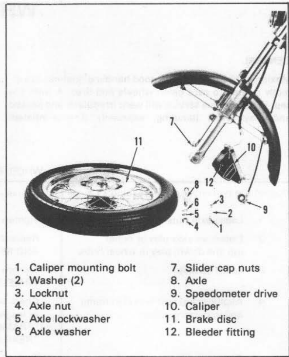
Figure 2-7. Front Wheel Removal (1974 to 1977)
