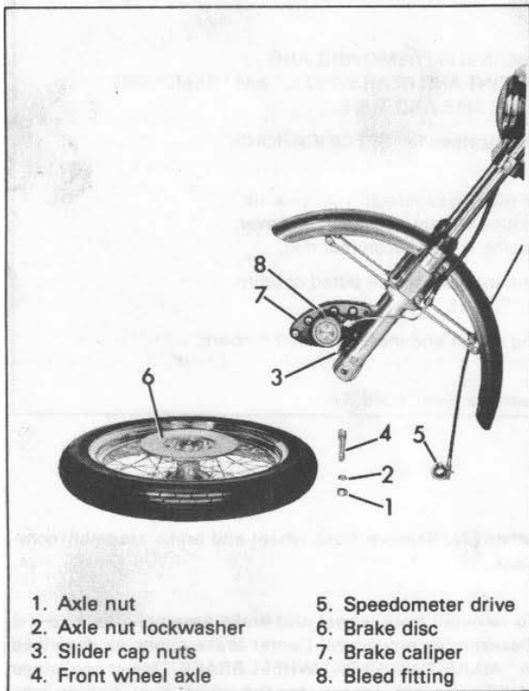
Figure 2-6. Front Wheel Removal (1973)
