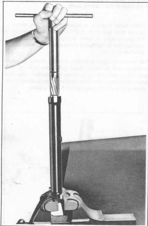
Figure 2-48. Reaming Fork Slider Bushing
