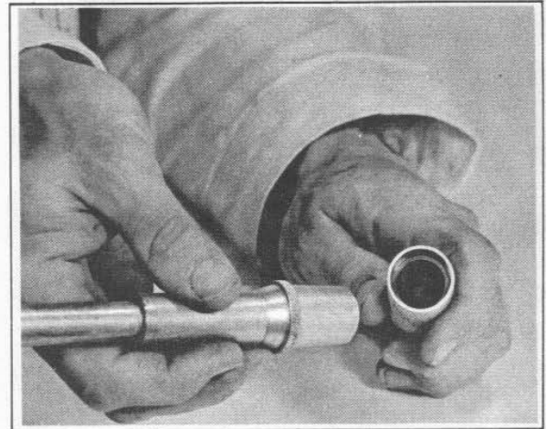
Figure 3-22. Inserting Piston Pin Lock Ring in Tool (1976 and Earlier)
