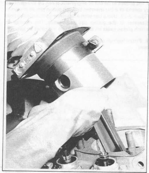
Figure 3-24. Installing Cylinder on Piston
