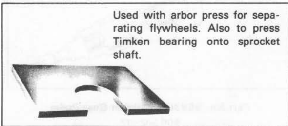
Part No. 96137-52A Flywheel Support Plate
