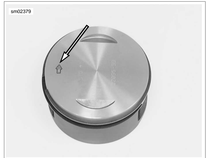
Figure 3-25. Piston Installation Arrow
