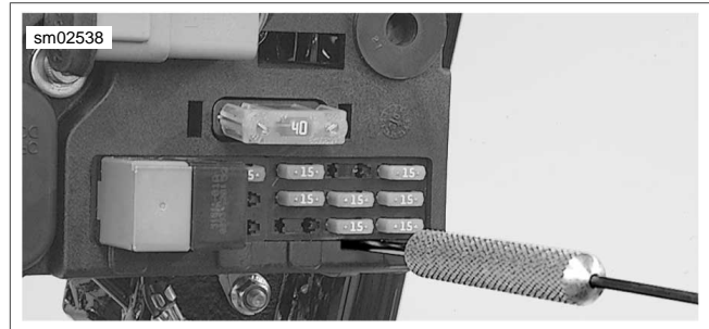
Figure 7-2. Removing Relay/Fuse Panels
