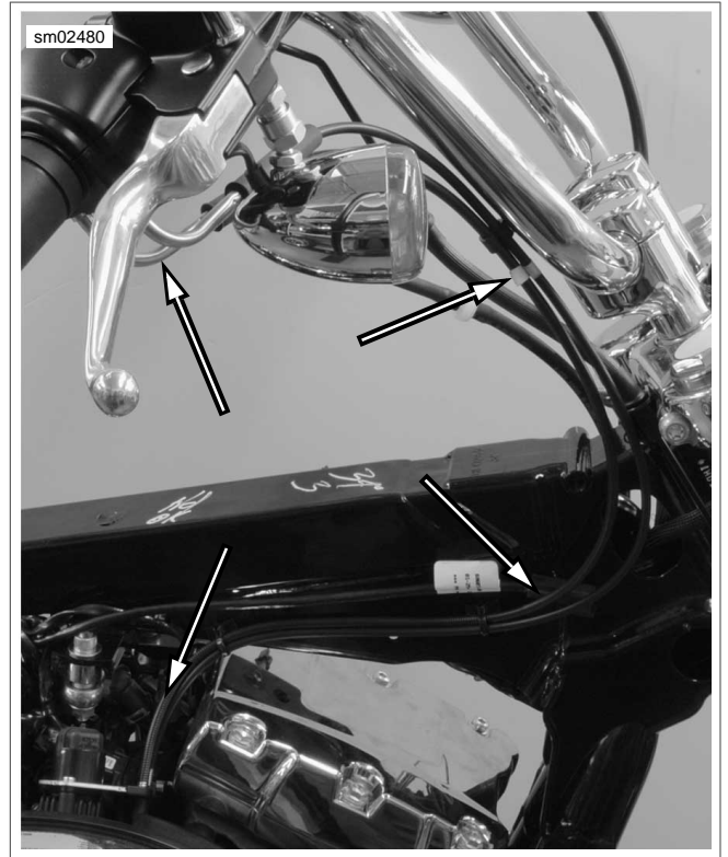
Figure 2-96. Throttle Cable Routing: FXDF (Typical)
