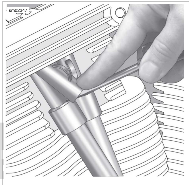
Figure 3-43. Install Spring Cap Retainers
