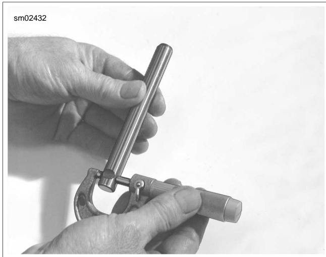
Figure 3-71. Checking Shaft to Support Plate Fit
