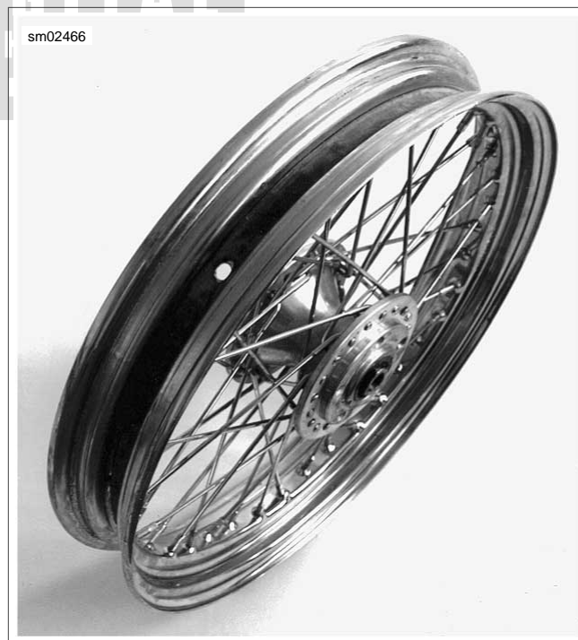
Figure 2-80. Installing Rim Strip
