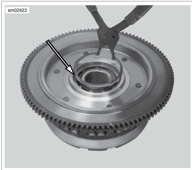
Figure 5-34. Install Clutch Shell Retaining Ring with Flat Side Against Bearing
