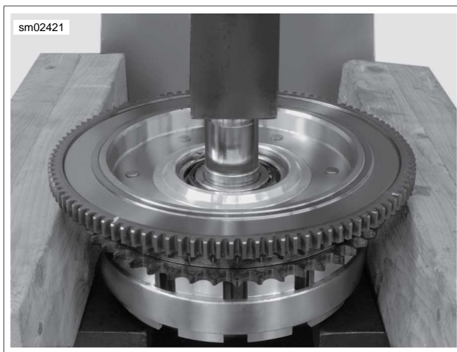
Figure 5-33. Pressing Clutch Hub From Bearing
