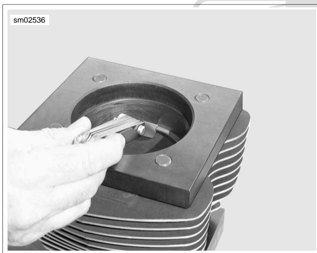
Figure 3-104. Measuring Ring Gap
