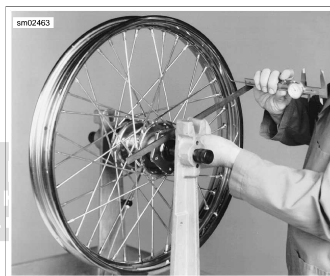
Figure 2-52. Front Wheel Hub Offset Dimension
