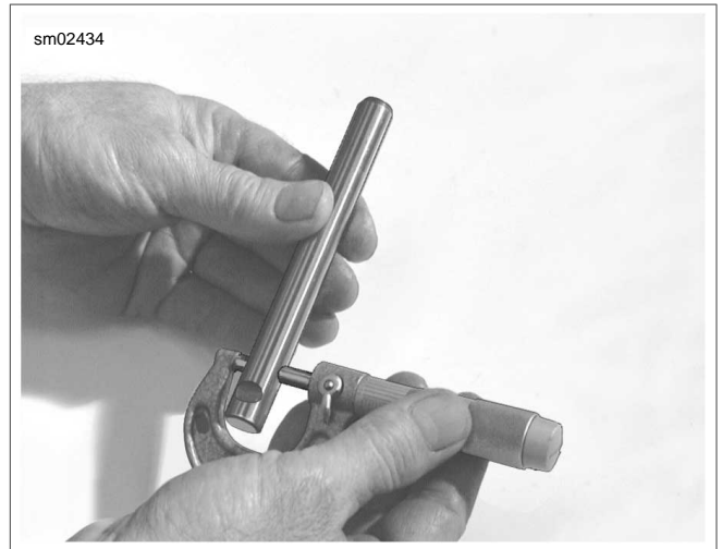
Figure 3-73. Checking Shaft to Bushing Fit
