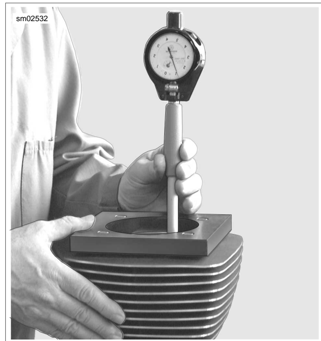
Figure 3-99. Measure for Out-of-Round and Taper
