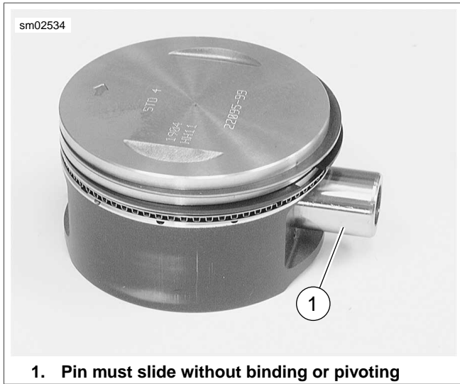
Figure 3-101. Piston Pin Clearance
