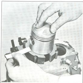
Figure 3C-11. Checking Rod Alignment
