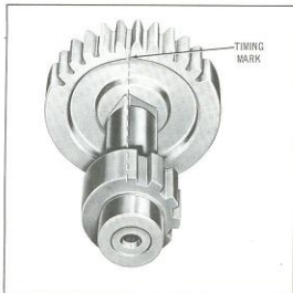
Figure 4D-7. Timing Shifter Gear
