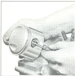
Figure 3C-2. Removing Piston Pin Lock Ring
