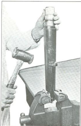
Figure 2F-17. Inserting New Oil Seal
