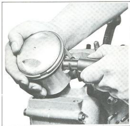
Figure 3C-14. Inserting Piston Pin Lock Ring
