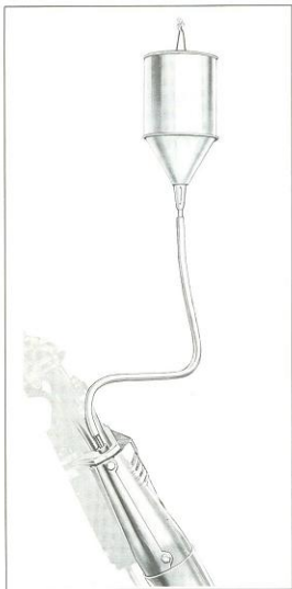
Figure 2F-2. Filling Hydraulic Fork with Oil
