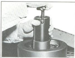
Figure 3E-7. Pulling Bearing from Sprocket Shaft
