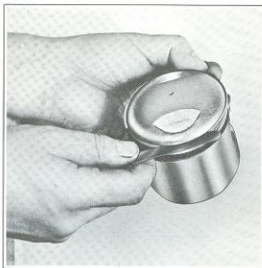
Figure 3C-6. Measuring Ring Side Clearance
