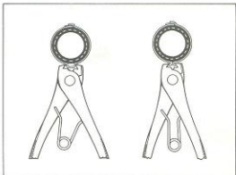
Figure 3D-1C. Hose Clamp Connection
