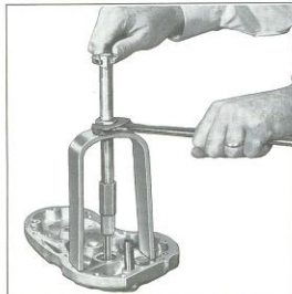
Figure 3D-6. Removing Pinion Shaft Cover Bushing
