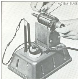
Figure 5E-4. Testing Armature for Short
