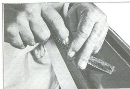
Figure 2J-4. Trimming Patch
