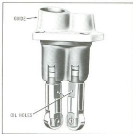
Figure 3D-3. Inserting Tappets on Guide
