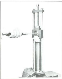
Figure 2F-19. Disassembling Shock Absorber (1966 & Earlier Shown)
