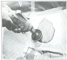
Figure 2J-13. Blending Patch with Sander
