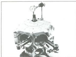
Figure 3E-17A. Checking Flywheel End Play
