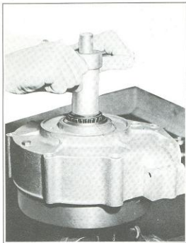
Figure 3E-17. Pressing Flywheel into Crankcase
