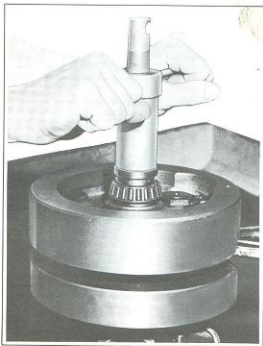
Figure 3E-16. Pressing Bearing on Sprocket Shaft
