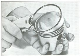
Figure 3C-9. Assembling Rings with Ring Expander
