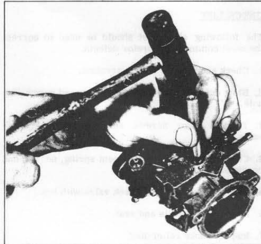
Figure 3F-7D. Removing Main Nozzle
