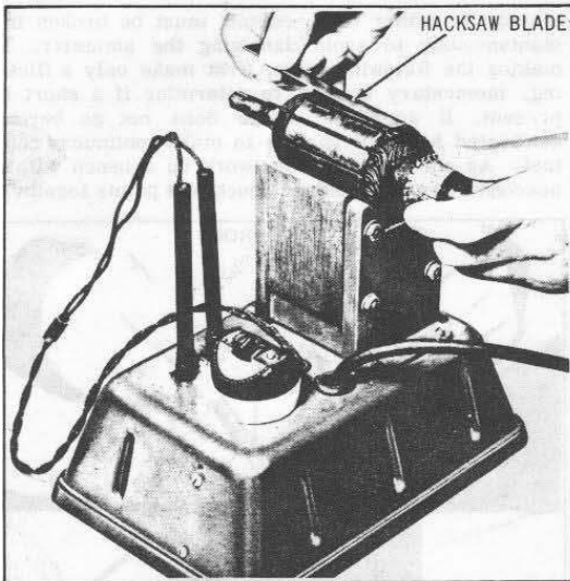
Figure 5E-4. Testing Armature for Short
