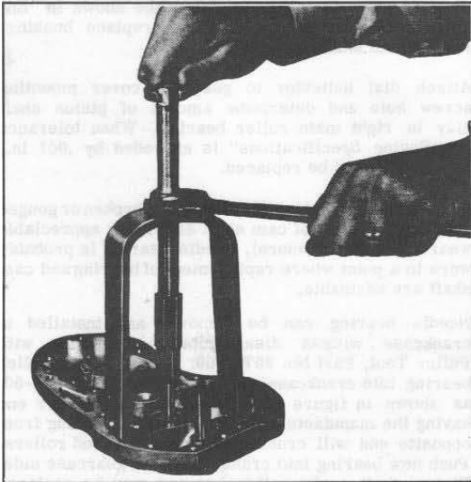
Figure 3D-6. Removing Pinion Shaft Cover Bushing
