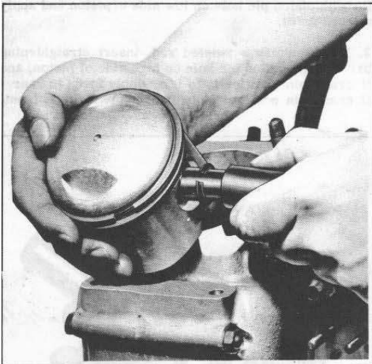
Figure 3C-14. Inserting Piston Pin Lock Ring
