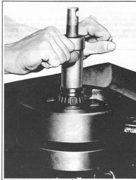
Figure 3E-16. Pressing Bearing on Sprocket Shaft
