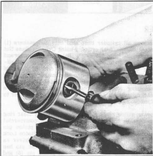
Figure 3C-2. Removing Piston Pin Lock Ring
