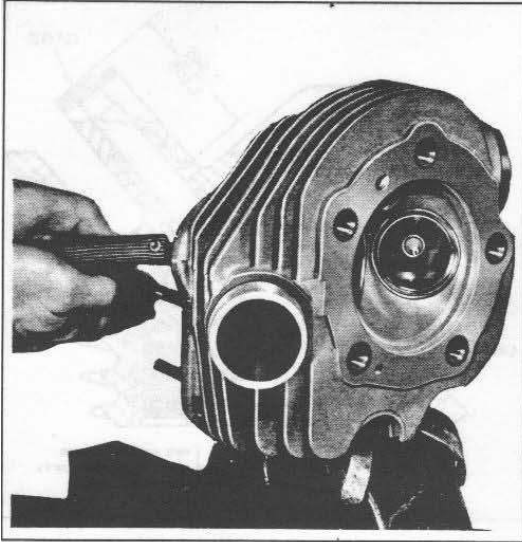
Figure 3B-4. Lapping Valves
