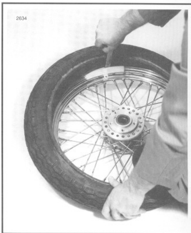
Figure 2-35. Starting Bead on Rim
