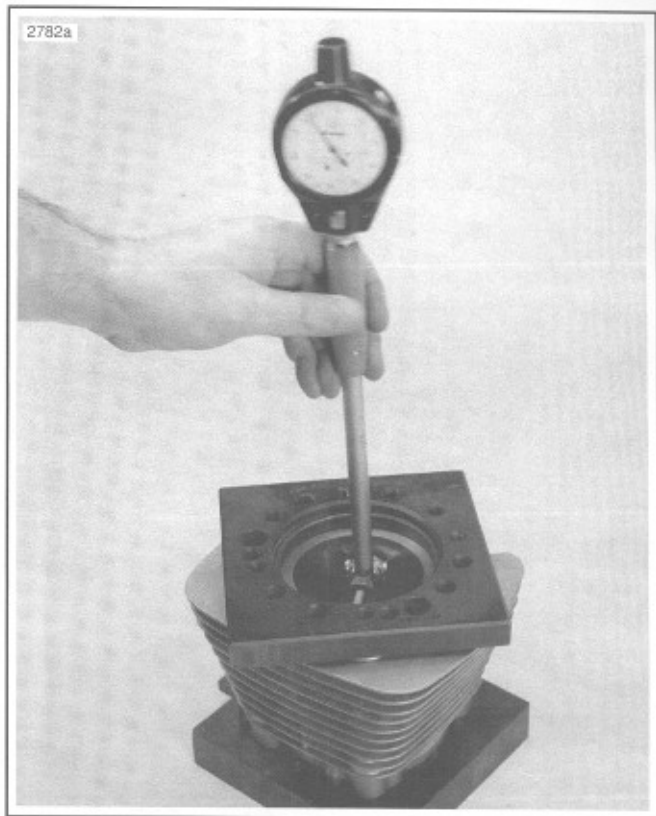
Figure 3-29. Measuring Cylinder Bore
