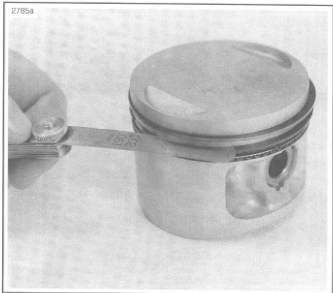
Figure 3-34. Measuring Ring Clearance in Groove
