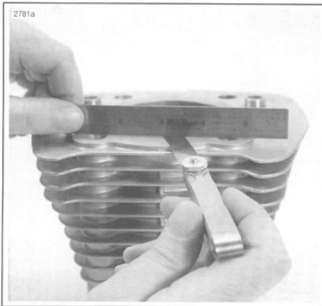
Figure 3-28. Checking Gasket Surfaces
