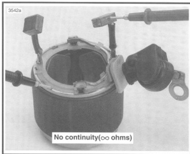
Figure 5-17. Grounded Field Test
