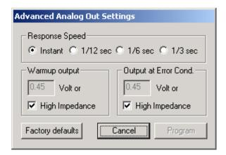
When setting the LM-1 to the slower response speed settings the measured mixture data will be averaged over the response time setting before being output.
