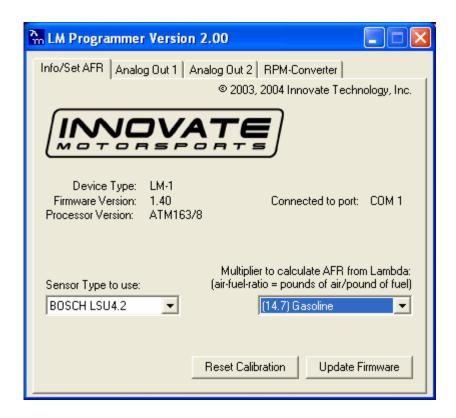
On this page you can see the software version of the LM-1, which sensor your LM-1 uses and you can change the multiplier to calculate AFR from Lambda. A number of different multipliers are already pre-selectable but you can change it to a custom one for the particular fuel you are using.
