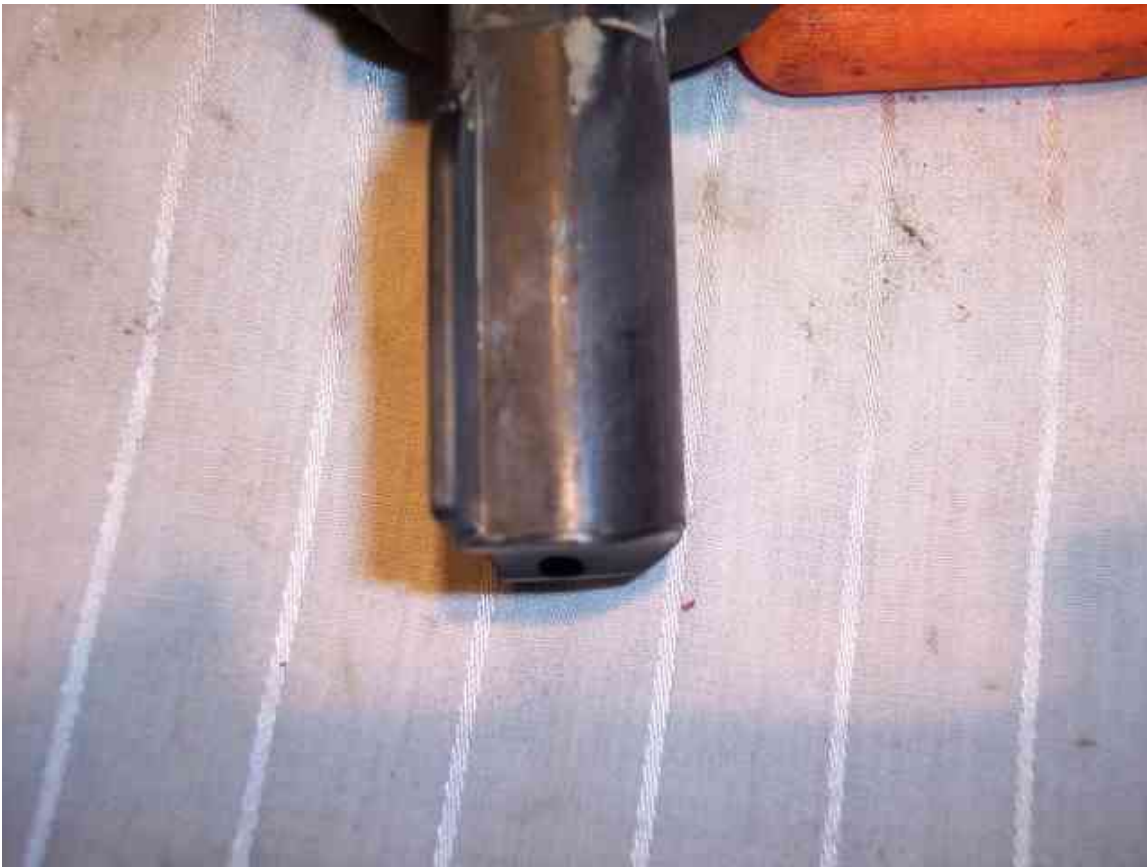
Side shot of the slide. The shape of the bottom of the slide is where the carbs get the "slingshot" term.
